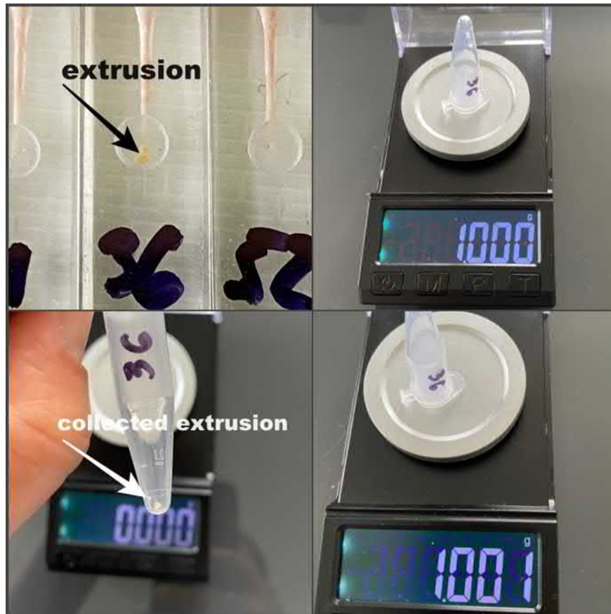
Fig. 5.: Measuring of extruded material, collected in Eppendorf tube. (source: author's own work)
