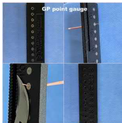
Fig. 3.: GP point gauge measuring if the end of the GP fits the size of the apical constriction accurately. The gauge pictured measures sizes from #20 to #140. (source: author's own work)
